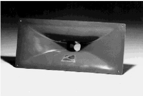
The CFD 1-100 Pro is a 1" entry throat, consistent "Q" horn with a functional frequency response of 1kHz to 16kHz. It has a particularly smooth frequency response across its 100°H x 52°V coverage pattern, which makes this horn an excellent choice for high quality reproduction in critical monitoring situations, or in high level foreground or small and medium club PA systems. Also available in a commercial model for low SPL applications.
