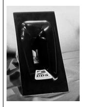
The CAD 2-954 Pro is our first release of the Continuous Asymetrical Distribution series from DDS. This horn is specifically designed to be used in an angled monitor face. The dispersion pattern is 90°H x 40°V in its near-field position and 50°H x 40°V at three meters. This allows for a high dB monitor level that develops an increasing "Q" in its down stage positions.
