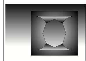
The DVB 15N Pro (shown as an illustration above) has an octagonal entry throat for a 15" cone type transducer for low and low-mid range reproduction. Its optimal range is 60Hz to 800Hz. At 15" deep this horn's nominal dispersion pattern is 70° x 70°. Designed to match the DMB 10N Pro or DMB 12N Pro in multi-way systems the DVB 15N is ideal for cluster configurations or to load the low end in medium to long throw club systems.
