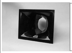
Based on the octagonal entry flare of our DVB 15H, the DMB 10N Pro is a mid-bass horn for a 10" cone type transducer. The DMB 10N Pro has a functional frequency response of 250Hz to 1.6kHz with a nominal dispersion pattern of 70°H x 60°V. The DMB 10N Pro is excellent for use in multiway sound systems and PA's with critical mid-bass requirements.
