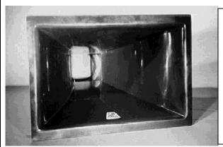
The DMB 10 is a straight exponential flare mid-bass horn with a nominal dispersion of 65° x 75° for a 10" cone type transducer. The DMB 10 has a functional frequency response of 250Hz to 1.5kHz. The DMB 10 is designed for reinforcement applications and used alone it is an excellent voice paging system in large outdoor or indoor areas. The DMB 10 is supplied with a compression cap of .6 cu. ft.
